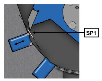
Fig. 30: Cutting gap
