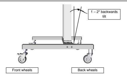
Fig. 16: Optimal alignment
