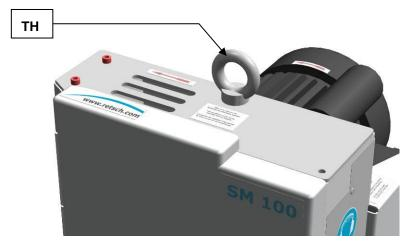
Fig. 2: Removing the transport aid
