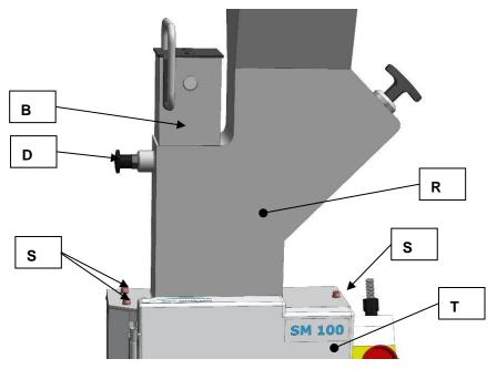
Fig. 14: Mounting the feed hopper
