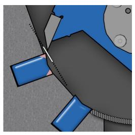
Fig. 26: Cutting gap
