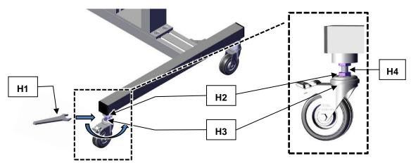
Fig. 15: Adjusting the height of the support structure
