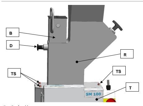
Fig. 33: Mounting the feed hopper
