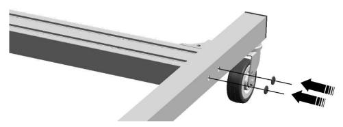
Fig. 7: Mounting the side protective caps
