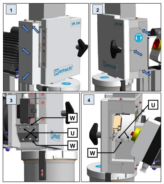
Fig. 27: Access to the cutting bars
