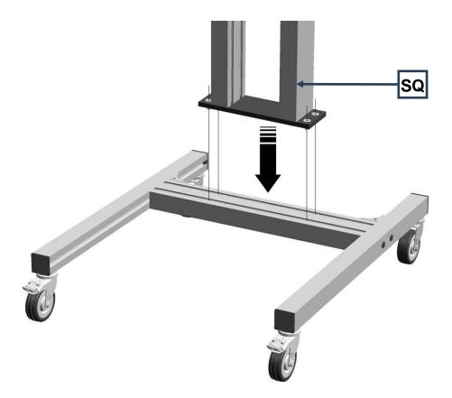
Fig. 9: Placing the crossbar on the stand
