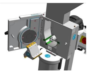
Fig. 34: Removing the rotor
