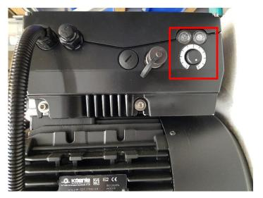
Fig. 18: Rotary control on the motor
