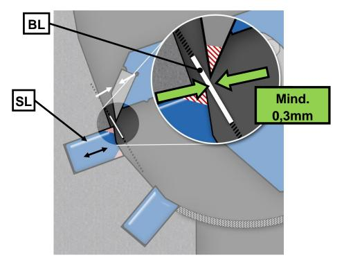
Fig. 29: Adjust the cutting gaps
