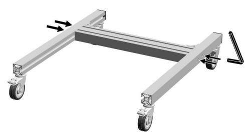
Fig. 6: Screwing the crossbar tight
