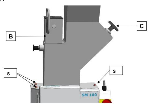
Fig. 31: Removing the feed hopper
