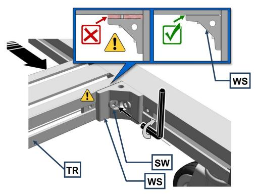
Fig. 5: Fastening the crossbar angle bracket
