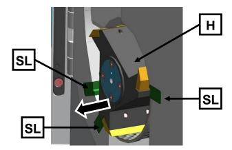
Fig. 28: Freely rotate the rotor
