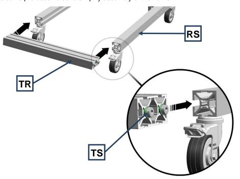
Fig. 4: Assembling the crossbar
