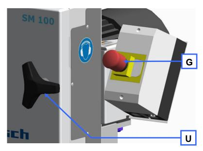
Fig. 21: Opening the grinding area door
