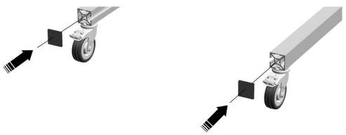
Fig. 8: Mounting the front protective caps
