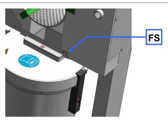
Fig. 35: Removing the discharge flange
