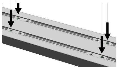
Fig. 10: Points for securing the stand
