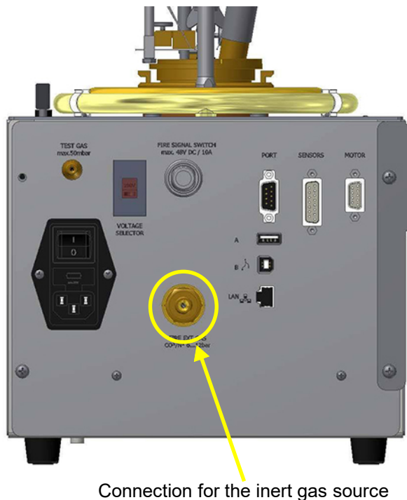
Fig. 3-6: Fire extinguisher system
